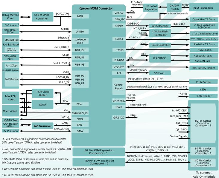
5 VI1 & VI2 can be used in 8bit mode. If VI1 is used in 16bit, then VI2 cannot be used.
