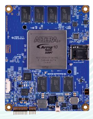
iWave's Arria 10 SoC System on Module is based on the Arria 10 SX family device with F34 package. The module is equipped with 32-bit DDR4 memory support for HPS with ECC and 64-bit DDR4 support for FPGA. All the IOs and high speed transceiver blocks will be available on the SOM board to board connectors.
