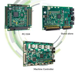
**Prodigy® Motion Boards** provide high performance board-level motion control for scientific, automation, industrial, and robotic applications. Available in PC/104, standalone, and machine controller configurations, these boards support multiple motor types including Brushless DC, step, and DC Brush motors, and are available in 1, 2, 3, and 4-axis configurations.
