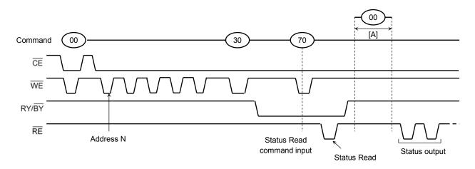
The device status can be read out by inputting the Status Read command "70h" in Read mode. Once the device has been set to Status Read mode by a "70h" command, the device will not return to Read mode unless the Read command "00h" is input during [A]. If the Read command "00h" is input during [A], Status Read mode is reset, and the device returns to Read mode. In this case, data output starts automatically from address N and address input is unnecessary.
