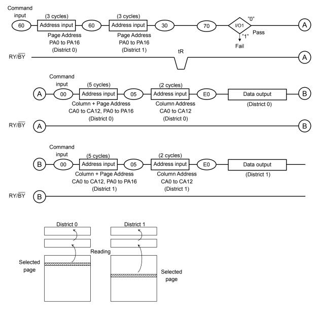
The data transfer operation from the cell array to the Data Cache via Page Buffer starts on the rising edge of  $\overline{WE}$  in the 30h command input cycle (after the 2 Districts address information has been latched). The device will be in the Busy state during this transfer period. After the transfer period, the device returns to Ready state. Serial data can be output synchronously with the  $\overline{RE}$  clock from the start address designated in the address input cycle.
