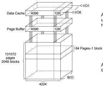
A page consists of 4224 bytes in which 4096 bytes are used for main memory storage and 128 bytes are for redundancy or for other uses.
