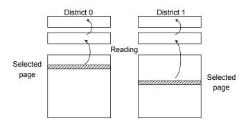
The data transfer operation from the cell array to the Data Cache via Page Buffer starts on the rising edge of  $\overline{WE}$  in the 30h command input cycle (after the 2 Districts address information has been latched). The device will be in the Busy state during this transfer period.
