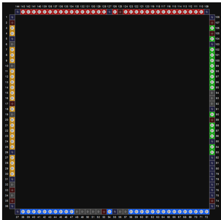
Figure 3-2 View of GW1NS-2/GW1NS-2C LQ144 Pins Distribution (Top View)
