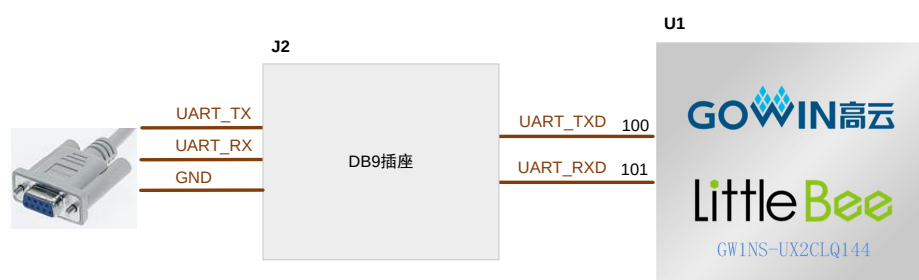
Figure 3-13 RS232 Download Connection
