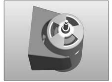
Step 2 A misalignment of the pin and the blind hole prevents proper installation of the probe.
