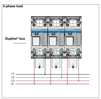
Note: The distance between the dimmer module and the light should not exceed 25 metres
