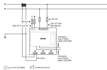
Fig. 3 Single-phase system with neutral (2-wire)
