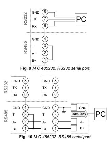
NOTE: additional meters with RS485 are connected in daisy chain. The serial output must only be terminated on the last network meter connecting terminals B+ and T.
