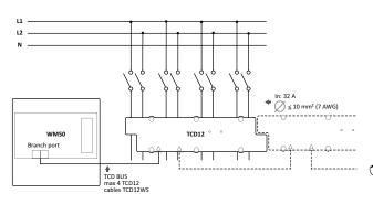
Fig. 13 Two-phase system with neutral (3-wire)
