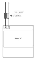
Fig. 12 Auxiliary power supply (H)
