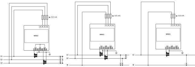
**Fig. 7** Three-phase without neutral (3-wire)
