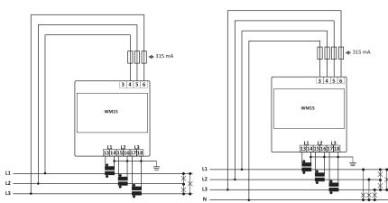
**Fig. 5** Three-phase without neutral (3-wire)
