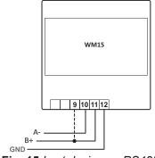
Fig. 15 Last device on RS485
