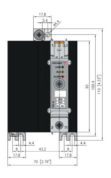
Housing width tolerance +0.5mm, -0mm as per DIN 43880.
