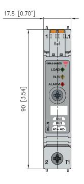
Housing width tolerance +0.5mm, -0mm as per DIN 43880. All other tolerances +/- 0.5mm.
