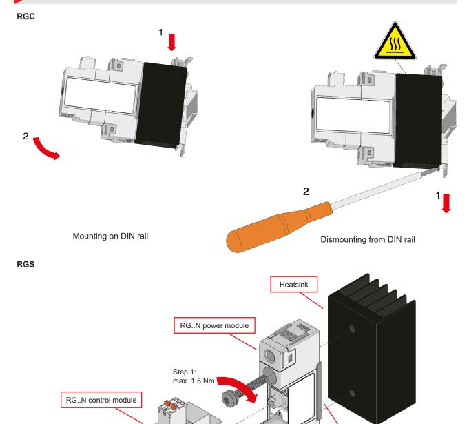
Step 1: Mount RG..N power module to Heatsink
