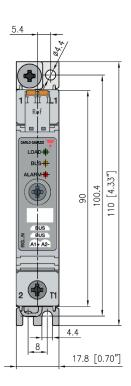
Housing width tolerance +0.5mm, -0mm as per DIN 43880.
