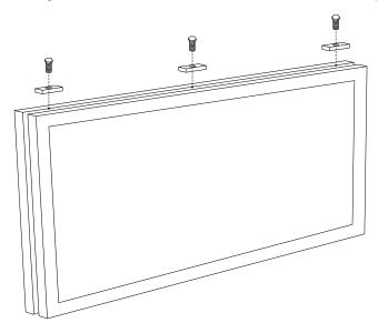
The display must be mounted by using the included hammer nuts.
