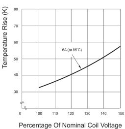
**Test conditions:** 6A 85℃ (Typical curve of 24VDC standard type)
