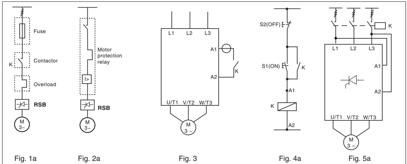
The motor controller provides by-passing of the semiconductors during running operation. Therefore the semiconductors can only be damaged by short-circuit currents during ramp-up and ramp-down. Please note that the motor controller does not insulate the motor from the mains.
