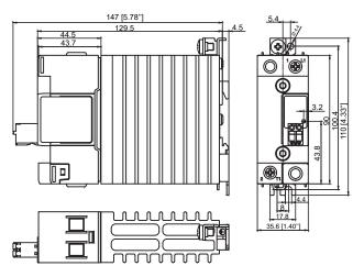
Housing width tolerance +0.5mm, -0mm as per DIN 43880. All other tolerances +/- 0.5mm. Dimensions in mm.
