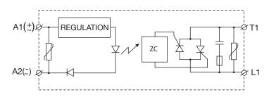
Note: Varistor on output is not included in the RGH1A69...models
