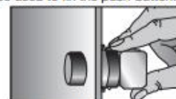
The contact block is snapped on.
