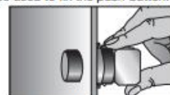
The contact block is snapped on.
