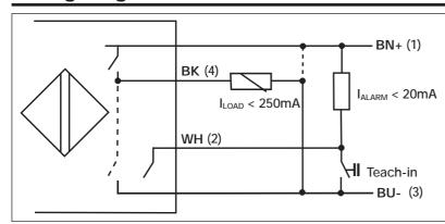
The PNP- or NPN-load will automatically be detected.
