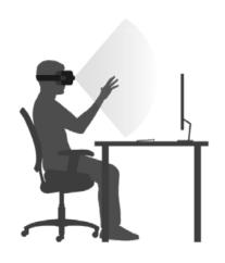
The Leap Motion Controller features a 140×120° field of view and an interactive tracking range of up to 60cm (24") or more.
