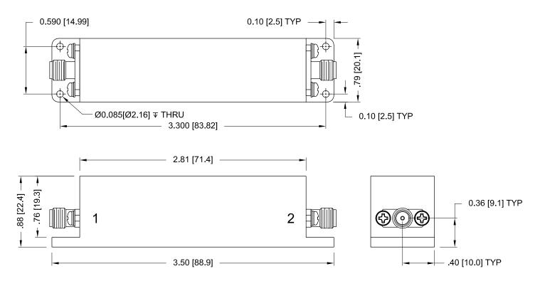
Unit Weight: 86 Grams. Dimensions are in inches (mm). Tolerances: 2 Pl. ± .100; 3 Pl. ± .015
