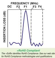
SMA-F ZVBP-4000-S+ Electrical Specifications at 25°C Parameter F# Frequency (MHz) Min. Тур. Max. Unit Center Frequency 4000 MHz 1 dB Bandwidth 6.0 MHz Pass Band Insertion Loss F1 4000 6.5 dB 4.5 VSWR F1 4000 1.3 1.5 •1 dB Insertion Loss DC-F2 DC - 3800 70 90 Stop Band, Lower VSWR DC-F2 DC - 3800 20 :1 Insertion Loss F3-F4 4200-6000 70 90 dB Stop Band, Upper 4200-6000 20 :1
