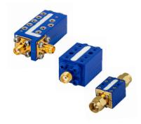
Mini-Circuits' Suspended Substrate Stripline filters offer low insertion loss by implementing printed circuit board suspended between two parallel ground planes, providing high Q. Low insertion loss combined with wide stopband makes them an excellent choice for wideband instruments and systems like ECM, ECCM, ELINT and ultrabroadband receivers.
