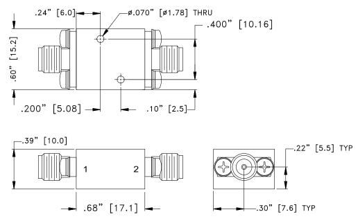
Unit weight: 24grams Dimensions are in inches (mm). Tolerances: 2 Pl.±.050"; 3 Pl.±.015"
