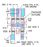
NOTES: 1. TRACE WIDTH IS SHOWN FOR ROGERS RO4350B WITH DIELECTRIC THICKNESS .020" ± .0015"; COPPER: 1/2 07. ON EACH SIDE. FOR OTHER MATERIALS TRACE WIDTH MAY NEED TO BE MODIFIED.
