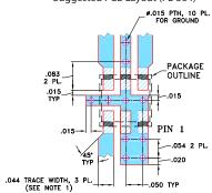
NOTES: 1. TRACE WIDTH IS SHOWN FOR ROGERS RO4350B WITH DIELECTRIC THICKNESS .020" ± .0015"; COPPER: 1/2 0Z. ON EACH SIDE. FOR OTHER MATERIALS TRACE WIDTH MAY NEED TO BE MODIFIED.
