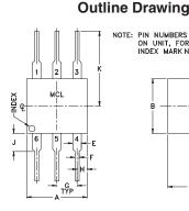
NOTE: PIN NUMBERS DO NOT APPEAR ON UNIT, FOR REFERENCE ONLY. INDEX MARK NEAR PIN 6.
