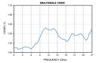
50Ω DC to 27 GHz SMA-Female Bulkhead to SMA-Female
