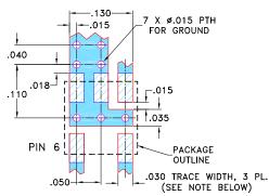
NOTE: 1. TRACE WIDTH IS SHOWN FOR ROGERS RO4350B WITH DIELECTRIC THICKNESS 0.030" ± 0.002"; COPPER: 1/2 OZ. EACH SIDE. FOR OTHER MATERIALS TRACE WIDTH MAY NEED TO BE MODIFIED.
