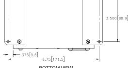
BOTTOM VIEW SHOWN WITH RUBBER FEET REMOVED AND BRACKETS INSTALLED.
