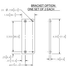
TOLERANCE: ±.005 INSTRUCTIONS FOR MOUNTING BRACKETS: TOOL REQUIRED: PHILLIPS HEAD SCREWDRIVER STEP 1: REMOVE RUBBER FEET FROM THE BOTTOM OF THE UNIT, DO NOT DISCARD THE FASTENERS. STEP 2: MOUNT THE BRACKETS WITH THE
