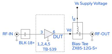
Fig 1. Block Diagram of Test Circuit used for characterization. (DUT soldered on Mini-Circuits Test Board TB-539+) Gain, Return loss, Output power at 1dB compression (P1 dB), Output IP3 (OIP3) and Noise Figure measured using Agilent's N5242A PNA-X microwave network analyzer.
