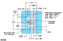
COPLANAR WAYEGUIDE PARAMETERS ARE SHOWN FOR ROGERS RO4350B WITH DIELECTRIC THICKNESS .010" ± .001". COPPER: 1/2 OZ. EACH SIDE. FOR OTHER MATERIALS TRACE WIDTH AND GAP MAY NEED TO BE MODIFIED.
