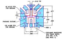
NOTES: 1. COPLANAR WAVEGUIDE PARAMETERS ARE SHOWN FOR ROGERS RO43508 WITH DIELECTRIC THICKNESS .010".2.001". COPPER: 1/2 02. EACH SIDE. FOR OTHER MATERIALS TRACE WOTH AND GAP MAY NEED TO BE MODIFIED 2. BOTTOM SIDE OF THE FOR IS CONTINUOUS GROUND FLANE.
