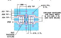
COPLANAR WAVEGUIDE PARAMETERS ARE SHOWN FOR ROGERS ROASSOB WITH THICKNESS .020° ± .0015°. COPPER: 1/2 OZ. EACH SIDE. FOR OTHER MATERIALS TRACE WIDTH & GAP MAY NEED TO BE MODIFIED. NOTES: 1.
