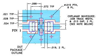
NOTES: 1. COPLANAR WAVEGUIDE PARAMETERS ARE SHOWN FOR ROGERS RO4350B WITH THICKNESS .020" ± .0015".
