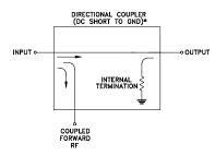
ELECTRICAL SCHEMATIC IS FOR DIRECTIONAL COUPLER WITH INTERNAL TRANSFORMER(S) THAT ROUTES DC FROM RF PORTS TO GROUND.
