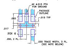
NOTES: 1. TRACE WIDTH IS SHOWN FOR ROGERS RO4350B WITH DIELECTRIC THICKNESS 0.030" ± 0.002"; COPPER: 1/2 0Z. EACH SIDE. FOR OTHER MATERIALS TRACE WIDTH MAY NEED TO BE MODIFIED.
