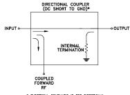
ELECTRICAL SCHEMATIC IS FOR DIRECTIONAL COUPLER WITH INTERNAL TRANSFORMER(S) THA ROUTES DC FROM RF PORTS TO GROUND.
