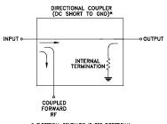
\* ELECTRICAL SCHEMATIC IS FOR DIRECTIONAL COUPLER WITH INTERNAL TRANSFORMER(S) THA
