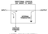
ELECTRICAL SCHEMATIC IS FOR DIRECTIONAL COUPLER WITH INTERNAL TRANSFORMER(S) THA BOULES DO ERROL BE RODTE TO CROWN TO
