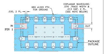
NOTE: 1. COPLANAR WAVEGUIDE PARAMETERS ARE SHOWN FOR ROGERS RO4350B WITH DIELECTRIC THICKNESS .060" ± .004";
