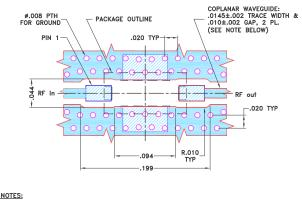
INULES: I. TRACE WIDTH PARAMETERS ARE SHOWN FOR ROGERS R04350B WITH DELECTRIC THICKNESS .0066"±.0007". COPPER: 1/2 02. EACH SIDE. FOR OTHER MATERIALS TRACE WIDTH AND GAP MAY NEED TO BE MODIFIED. 2. BOTTOM SIDE OF THE PCB IS CONTINUOUS GROUND PLANE. DENOTES PCB COPPER LAYOUT WITH SMOBC (SOLDER MASK OVER BARE COPPER). DENOTES COPPER LAND PATTERN FREE OF SOLDER MASK.
