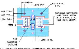
NOTES: 1. COPLANAR WAVEGUIDE PARAMETERS ARE SHOWN FOR ROGERS R04350B WITH THICKNESS .020" ± .0015". COPPER: 1/2 OZ. EACH SIDE. FOR OTHER MATERIALS TRACE WIDTH & GAP MAY NEED TO BE MODIFIED.
