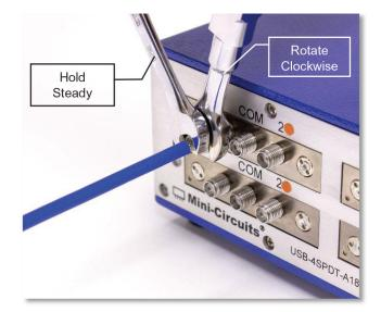
\*NOTE: Mini-Circuits recommends using a 5/16-inch open end wrench calibrated to 8 inch-pounds maximum torque to prevent damage due to over-torqueing the connector.
