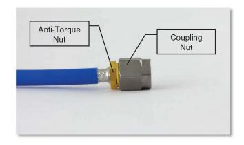
2) To properly tighten the cable, use a standard 1/4-inch open end wrench to brace the anti-torque nut.
