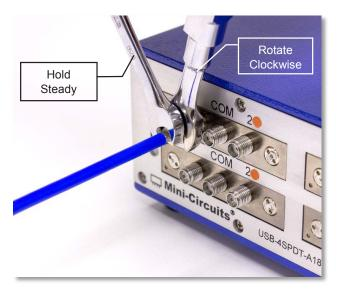
\*NOTE: Mini-Circuits recommends using a 5/16-inch open end wrench calibrated to 8 inch-pounds maximum torque to prevent damage due to over-torqueing the connector.
