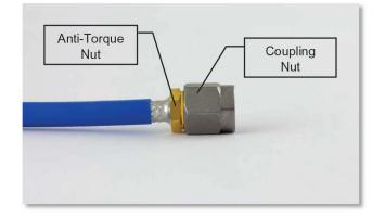
2) To properly tighten the cable, use a standard 1/4-inch open end wrench to brace the anti-torgue nut.
