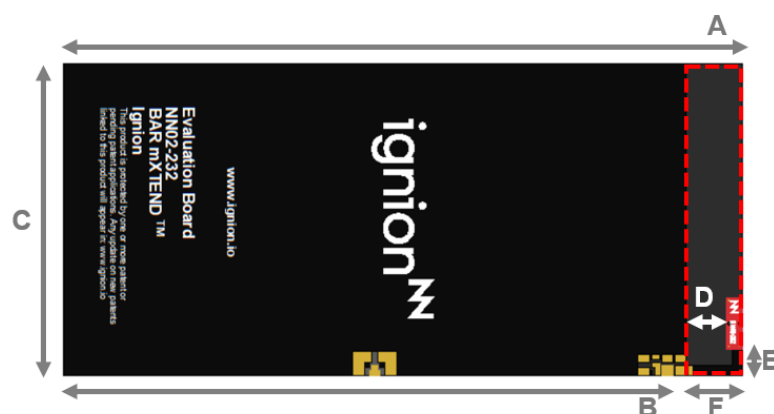
Figure 1 – EB_NN02-232-1B-2R-1P. Evaluation Board providing operation from 824 MHz to 960 MHz and from 1710 MHz to 2170MHz.
