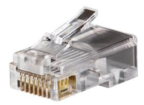
Klein's data and telephone plugs are professional-grade and deliver consistent, reliable performance. Our thick 50 micro-Inch gold plating on contacts prevent erosion and extended connector life. The three-pronged contacts provide more reliable connections with solid and stranded wire. The plug is housed in a durable resin with a spring clip. Expect a sure connection each and every time.
