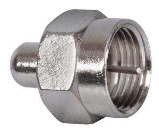
The F-Terminator is designed to terminate RF signals on unused equipment ports. It prevents extraneous signals from decreasing system performance. The F-Terminator also has a high return loss for improved signal quality.
