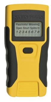
This compact cable tester is an easy-to-use tester that saves time and money on the job. The LAN Scout® Jr. tests continuity on twisted pair data wiring connections. An integrated tone generator supports multiple tones and control of the pins carrying the tone. The self-storing remote makes this tool easy to store and locate.
